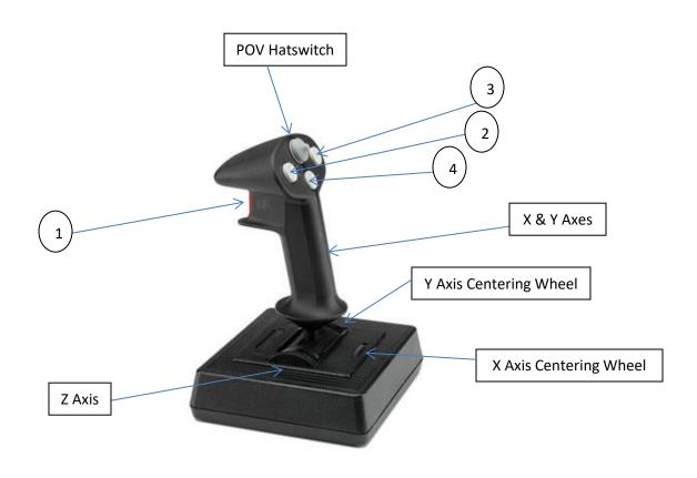
X Axis = Joystick Handle Turning Left and Right. In FS2020, assign "Ailerons Axis" to "Joystick L-Axis X"
